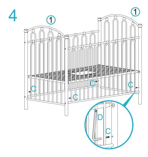
Place 4x short bolts (C) into the spare holes on both panels [1] as shown, and tighten with an allen key. Ensure the bolts are 100% tight before use. Lift furniture into the desired location, do not drag. You're done, enjoy!
