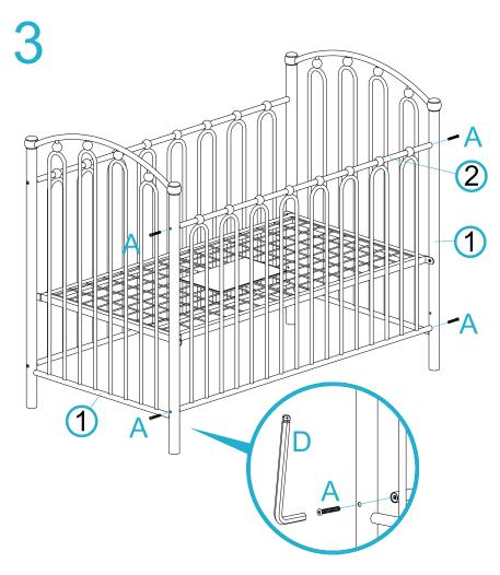
Attach side panel [2] to end panels [1] using 4x long bolts (A) and tighten with the allen key (D).
