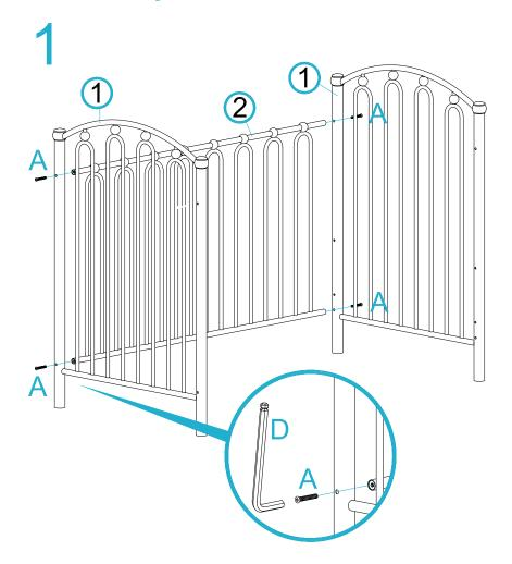
Attach the end 2x panels [1] to side panel [2] using 4x long bolts (A) and secure with the allen key (D).
