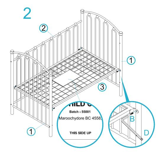
Attach base panel [3] to the rest of the frame using 4x medium bolts (B) and tighten with the allen key (D) as shown. Ensure you follow the directions for the correct mattress support height for your child on Page 2.
